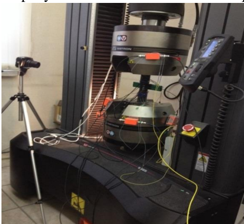
Fig. 1 Stretching - tensile machine "INSTRON-250"
