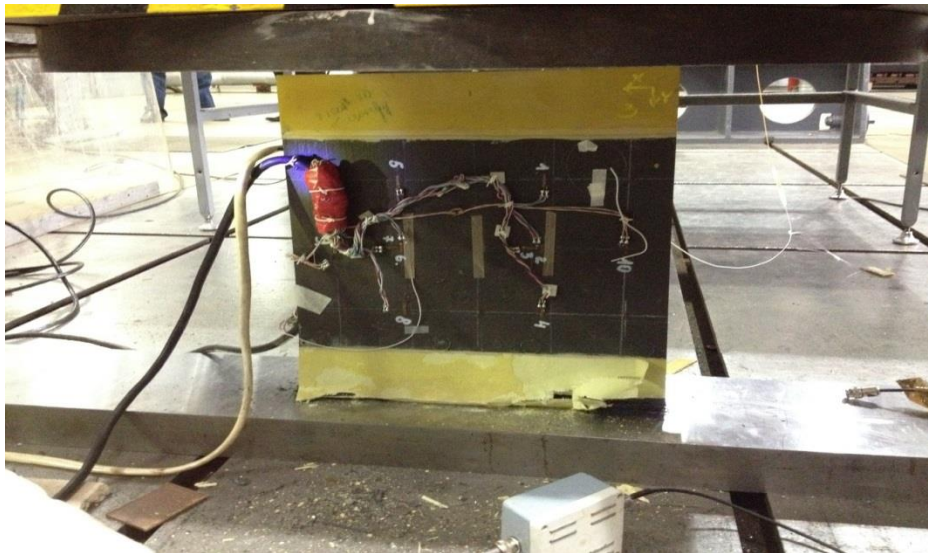
Fig. 5 Specimen of PCM installed between units of compression machine
